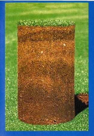
The best way to analyze physical properties is through undisturbed core analysis. By using 2" X 4.5" cores that are sealed in airtight copper tubes, your turf-intact core arrives at the ISTRC lab undisturbed.
